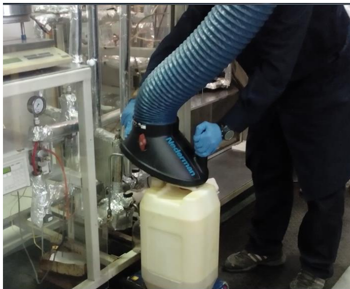
Figure 49 The loaded feed tank of a CETH/CPERI pilot plant
