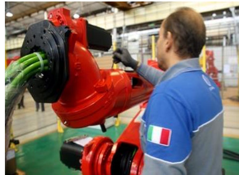
Figure 24 COMAU Final assembly of the robot arm
