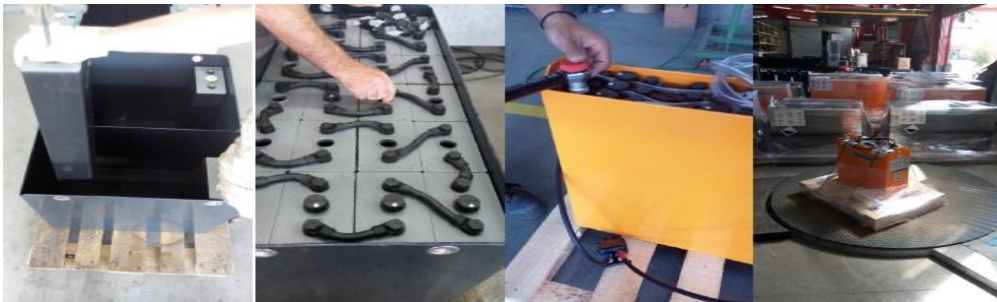
Figure 42 Battery assembly procedure at SUNLIGHT
