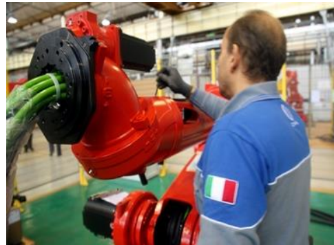
Figure 24 COMAU Final assembly of the robot arm
