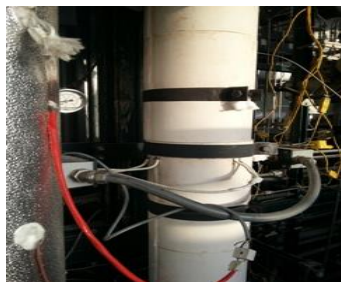
Figure 48 Part of a reactor, including a heating resistance at CERTH/CPERI
