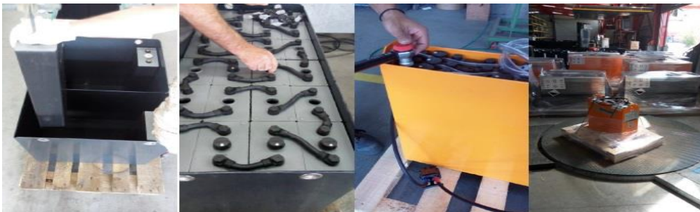
Figure 42 Battery assembly procedure at SUNLIGHT
