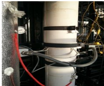
Figure 33 Part of a reactor, including a heating resistance at CERTH/CPERI
