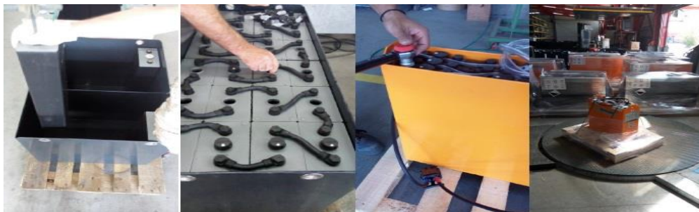
Figure 30 Battery assembly procedure at SUNLIGHT
