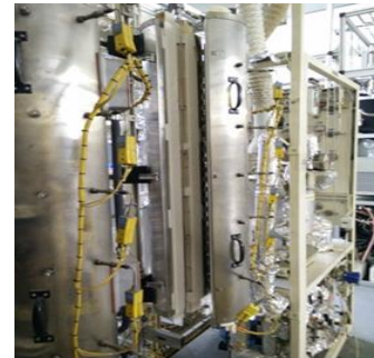
Figure 34 An unloaded and a loaded reactor at a CERN/CPERI pilot plant
