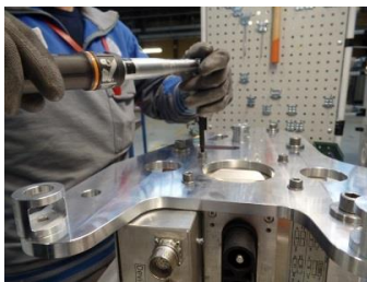
Figure 26 COMAU welding gun body assembly (a)
