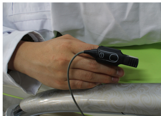
Fig. 3 Photoplethysmogram transducer
