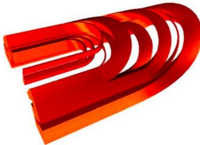
Figure 1: Optimized design of the SIS300 dipole cos-theta-coil [3]. The different bending radii of the cable depending on the position of the cable in the winding pack is clearly visible.
