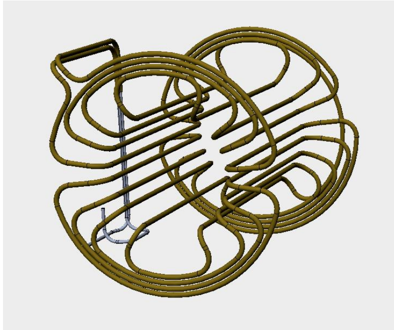
Figure 2: The coil layout depicts one coil of a nested SIS100 steerer coil. The primary coil layout follows that of a cos-theta magnet, but the coil heads are designed differently from the classical cos-theta design. This modification is necessary because two steerer magnets are nested into each other for this magnet, combining both horizontal and vertical steering capabilities.
