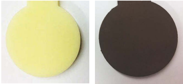
Figure 1: Test samples according to ISO 7619-1:2010 with 6 mm thickness and 5 cm diameter: uncoated sample (left) and Ag/AgCl coated sample (right).
