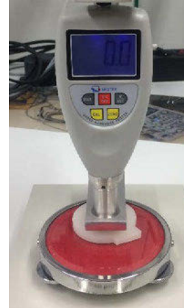
Figure 2: A test sample is placed on the stand hardness tester.
