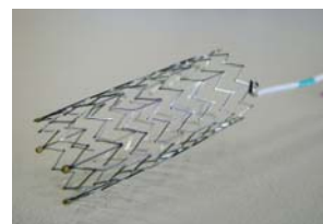
Fig. 1 Single wire soldered at a stent
