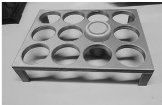
Figure 1. Adapter designed in 3D to be incorporated into a thermostatic bath.
