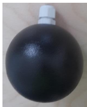
Figure 7: Black globe for operative temperature measurements using the Pt100 sensors.
