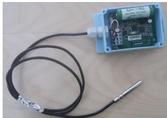
Figure 6: Pt100 with wireless transmitter used in the experiment.
