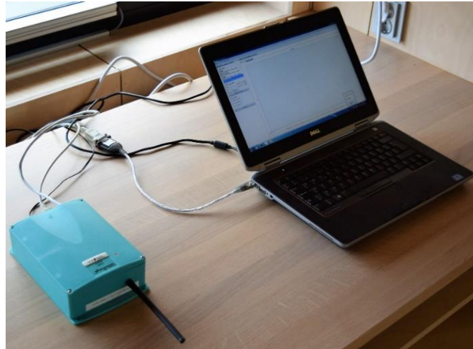
Figure 5: Wisensys base station setup for the data collection from the Pt100.
