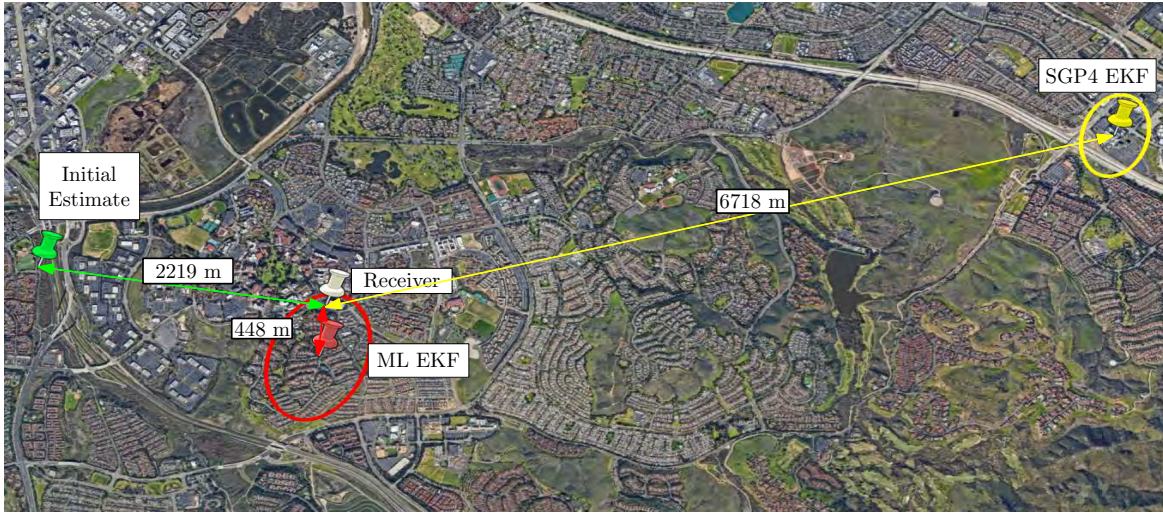
Fig. 9. Experimental results showing the initial and final 2-D stationary receiver localization errors and associated 95% uncertainty ellipses using (i) SGP4-propagated ephemeris and (ii) ML-propagated ephemeris. Map data: Google Earth.
