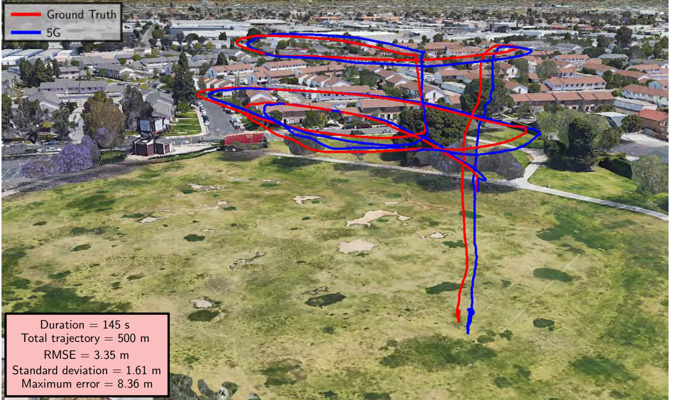
Fig. 5. The 5G navigation solution exhibited a position RMSE of 3.35 m versus the ground-truth reference navigation solution. Image: Google Earth.
