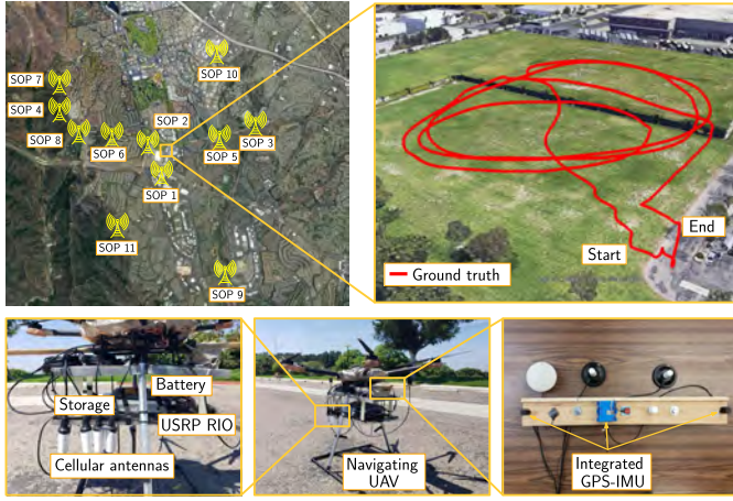
Fig. 14. Experimental hardware setup and the traversed trajectory along with the position of cellular LTE SOP towers.
