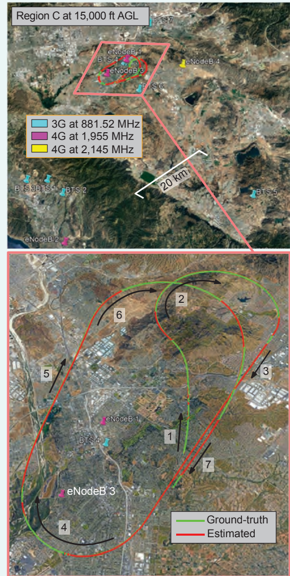
FIG 10 Experimental layout and results in Region C showing BTS and eNodeB positions, true aircraft trajectory, and aircraft trajectory estimated exclusively using cellular SOPs. The aircraft traversed a total distance of 55 km in 8.5 min during the experiment. The position RMSE over the entire trajectory was found to be 15.44 m.
