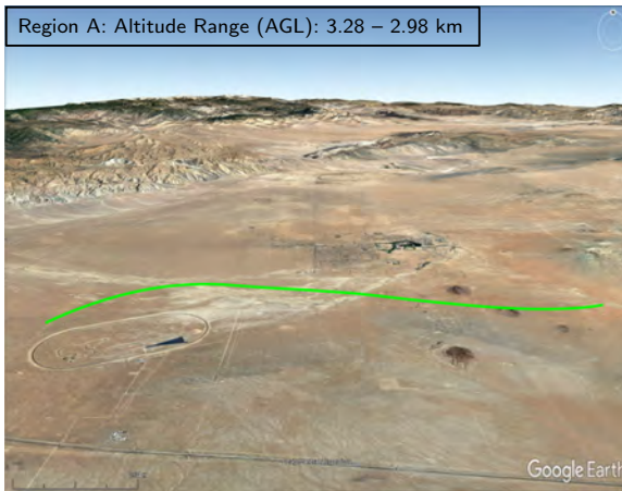
Figure 6: Left: descending teardrop aircraft trajectory in Region A. Right: receiver's pseudorange and Doppler tracking results from cellular LTE eNodeBs during this trajectory along with the C/N_0 and number of tracked eNodeBs.
