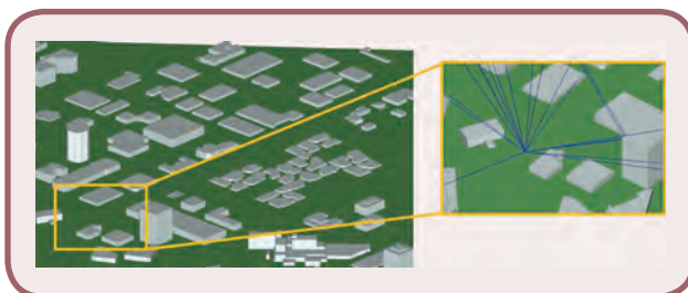
FIG 4 The ray tracing at a single node within a 3D urban digital map.
