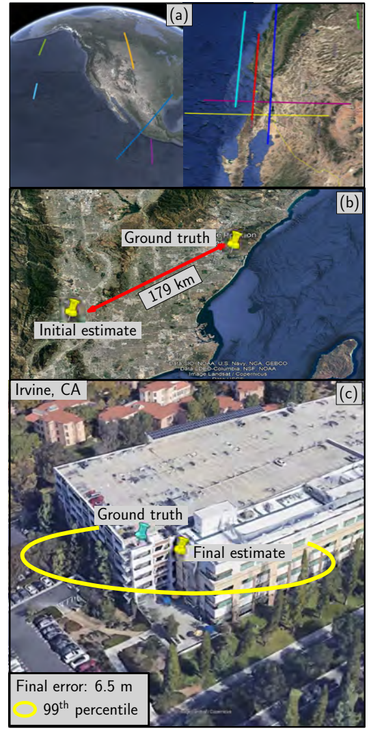
Fig. 2. (a) Trajectories of 11 LEO satellites (6 Starlink, 1 Orbcomm, and 4 Iridium NEXT) used to localize the stationary receiver. (b) Initial and final estimated positions. (c) Final errors relative to the receiver's true position.
