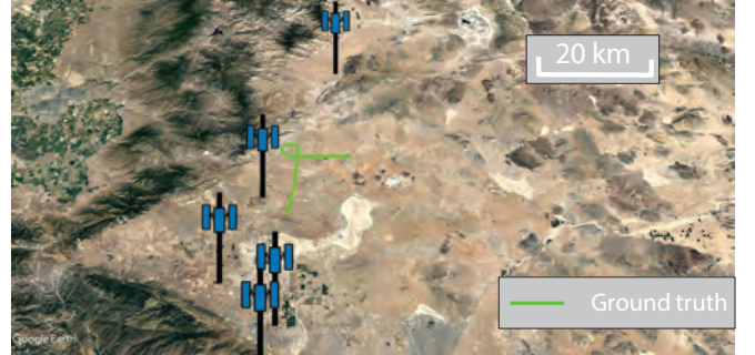
Fig. 1: Experimental environment in region A showing the aircraft trajectory and the locations of the 5 LTE eNodeBs.
