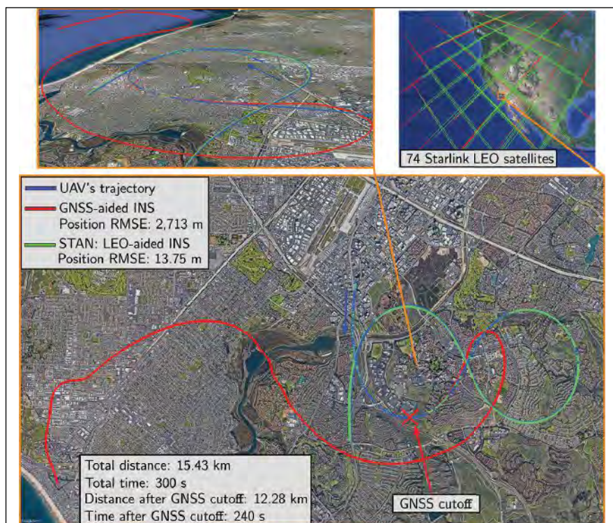
FIGURE 18 Simulation results of a UAV traveling 15.43 km in 300 seconds, where the last 240 seconds are without GNSS signals.
