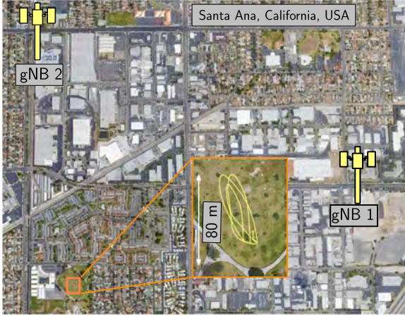
Fig. 8. Environment layout and UAV trajectory for the 5G NR UAV experiment.
