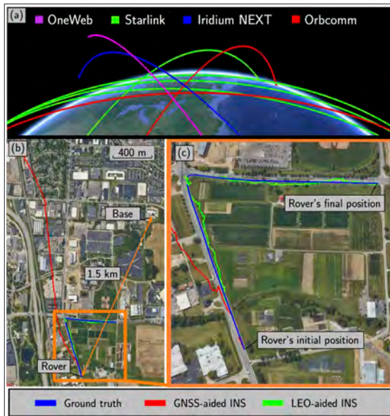
FIGURE 10 (a) LEO satellite trajectories of 4 Starlink, 1 OneWeb, 2 Orbcomm, and 1 Iridium LEO satellites whose signals were exploited for ground vehicle navigation, (b) relative distance between the base and rover (ground vehicle), (c) navigation results: ground truth trajectory (blue), GNSS-aided INS (red), and DSTAN LEO-aided INS (green).
