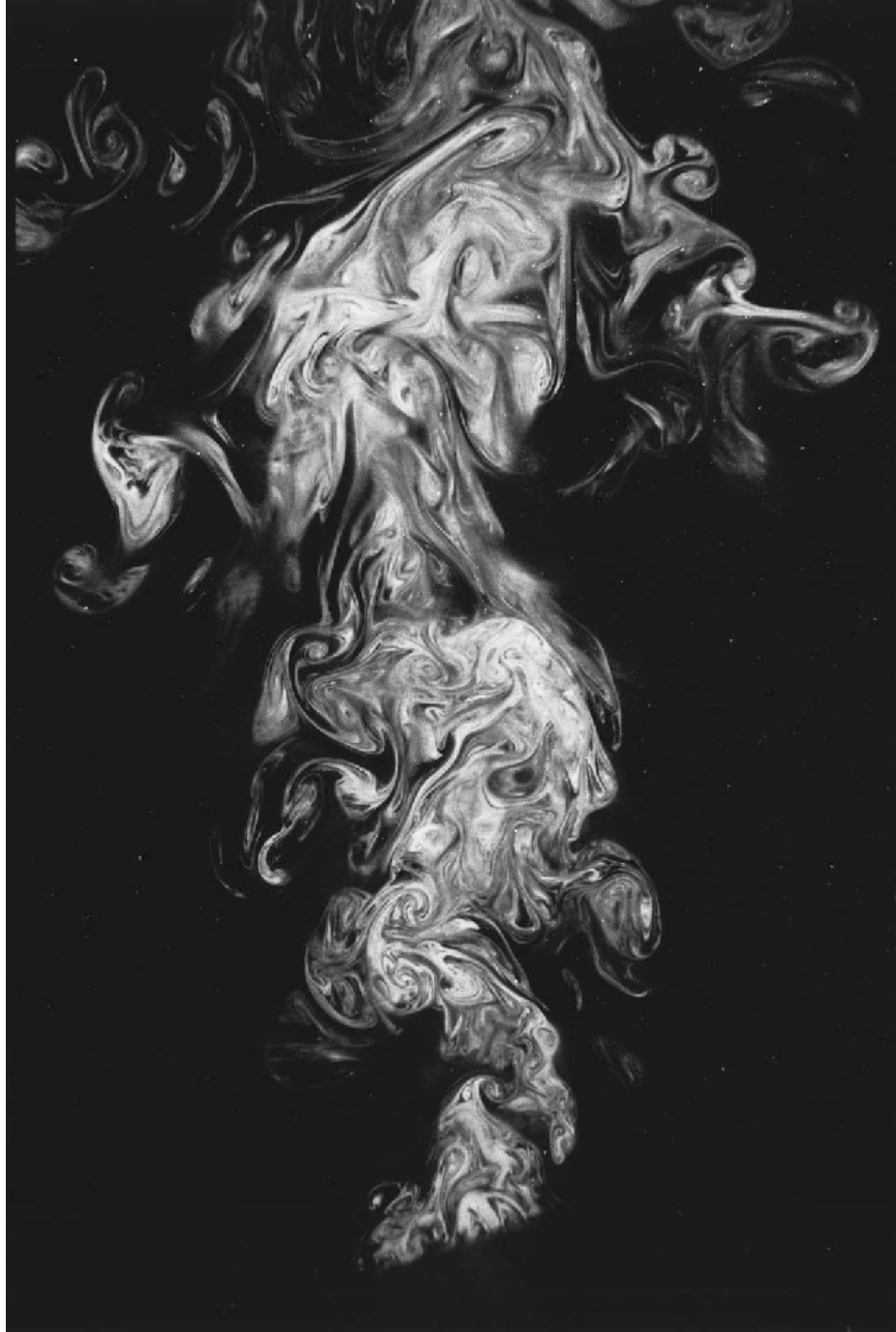
Figure 2.1: Turbulent eddies visualized in a tank of water via the addition of fluorescent dye and illuminated with a thin light sheet (Sreenivasan, 1999).
