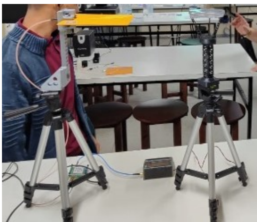
Figure 2 - Assembly made to irradiate microwave signals in the culture to be irradiated.
