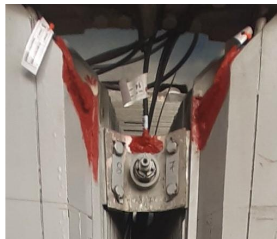
Figure 3. A detail of installed temperature sensors
