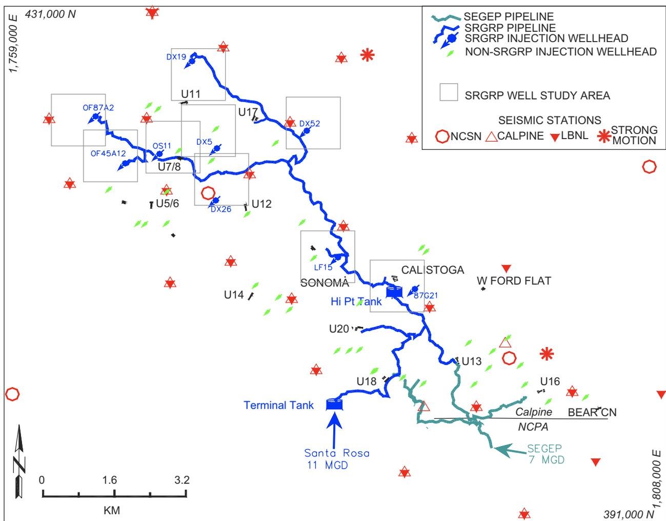
Fig. 2. Location of USGS (NCSN) stations, current Calpine array (pen triangles), and the first phase of the new stations (solid inverted triangles). Also shown are the locations of the pipelines used for the water from Santa Rosa. And the pipeline installed prior to this study in 1997 to inject water into the southeast Geysers (SEGP) at a rate of 26 million liters/day (7 million gallons/day, from [18]).
