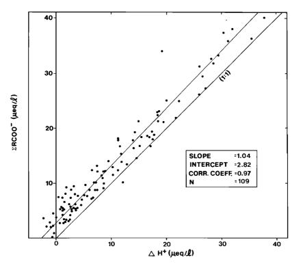
Fig. 2. The relationship between the  $\Sigma RCOO^-$  (HCOO<sup>-</sup> + CH<sub>3</sub>COO<sup>-</sup>) and  $\Delta H^+(H_{field}^+ - H_{lab}^+)$  in all samples with sufficient data.
