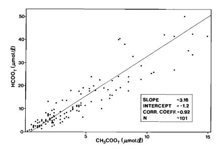
Fig. 10. Reduced major axis regression of  $HCOO_T$  versus  $CH_3COO_T$  in samples of precipitation collected at Katherine, Australia.
