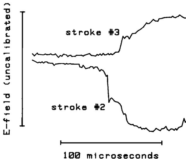
Fig. 2. NSSL fast antenna recording system electric-field waveforms (uncalibrated) of the second and third strokes in the triggered flash of Figure 1. The 10-90% risetime of the fast antenna was  $0.5 \mu\text{s}$  with a decay time of 1 ms.
